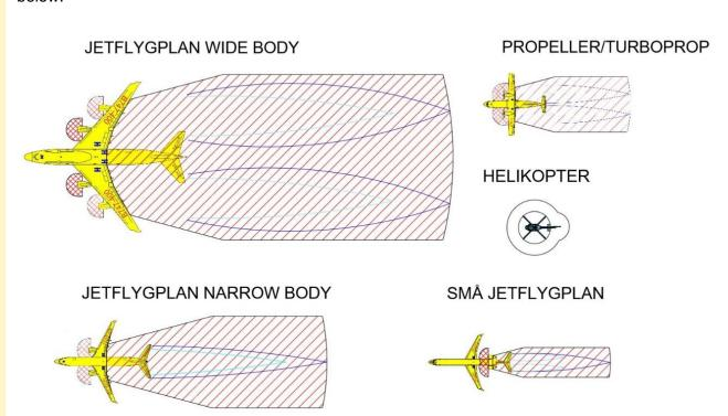
The distance of the risk area to the aircraft is defined by the aircraft manufacturer. Due to risks associated with jet blasts and of being sucked into an engine, these risk zones must be considered when around an aircraft.
