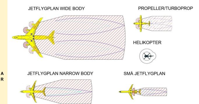
The distance of the risk area to the aircraft is defined by the aircraft manufacturer. Due to risks associated with jet blasts and of being sucked into an engine, these risk zones must be considered when around an aircraft.
